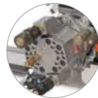
Main motor with leak-oil connection
