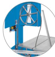
Fast, simple saw band replacement thanks to quick-release fastener
