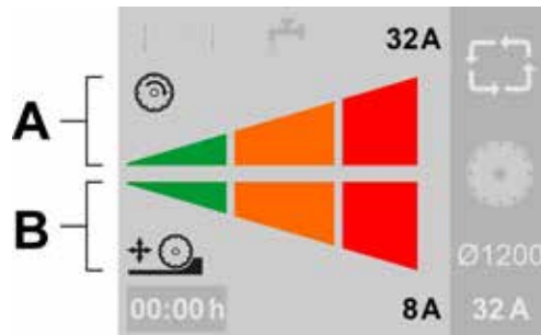
Display of the power for the feed- and main motor
